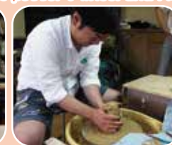
Making shapes: softening soil like mud, putting it on the center of hand and electric potter's wheel and making shapes finally
